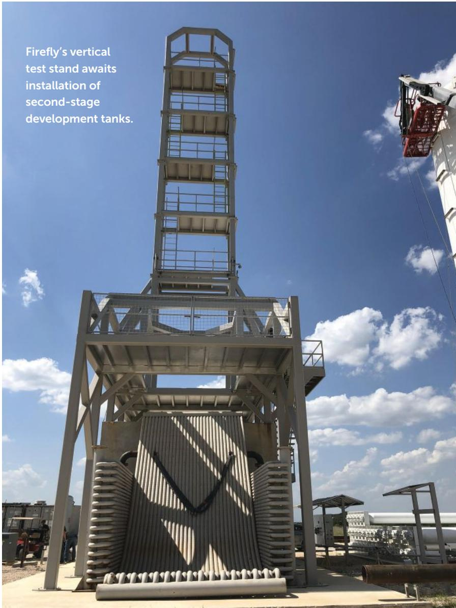
Firefly's vertical test stand awaits installation of second-stage development tanks.
