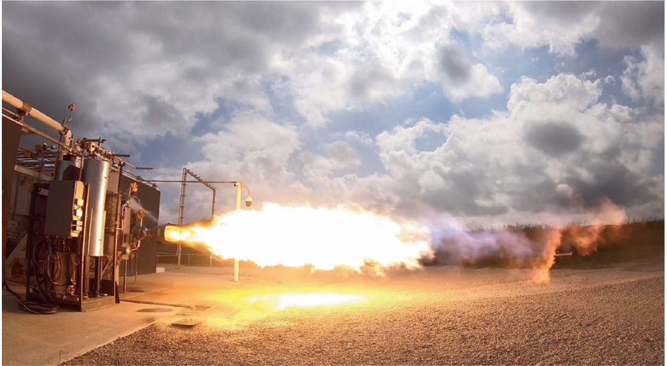
One of the four Reaver engines that power the Firefly Alpha's first stage undergoes a short-duration test at the company's Briggs, Texas, development facility.
